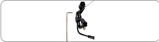
7. Pull the cable until it is tight and fix the screw with 2mm allen key.
