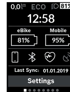
As well as the status bar, the status page also shows you the current time and the state of charge of all your eBike's batteries, as well as the state of charge of your smartphone battery if the smartphone is connected via Bluetooth®. It may also display symbols to indicate an activated Bluetooth® function or a device connected via Bluetooth® (e.g. a heart-rate monitor). You will also be shown the date of the most recent synchronisation between the smartphone and Kiox.
