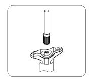
Use a compatible shock pump and adjust to your desired pressure.
