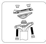
Disassemble all of the clamps from the top head of the post.
