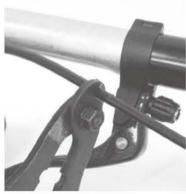
Cut the cable housing at a position where it reaches the top mount lever clamp on the side that is furthest away from the center of the handlebar (see photo).
