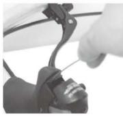
Detach the brake cable from the brake as per manufacturer's direction.
