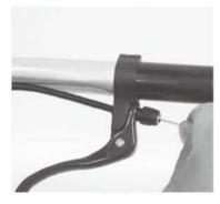
Re-insert the original bake cable through from the drop down handlebar lever,
