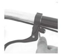
Open the hinged clamp of the top mount lever by-unscrewing the clamping bolt-with a 4mm Allen key.
